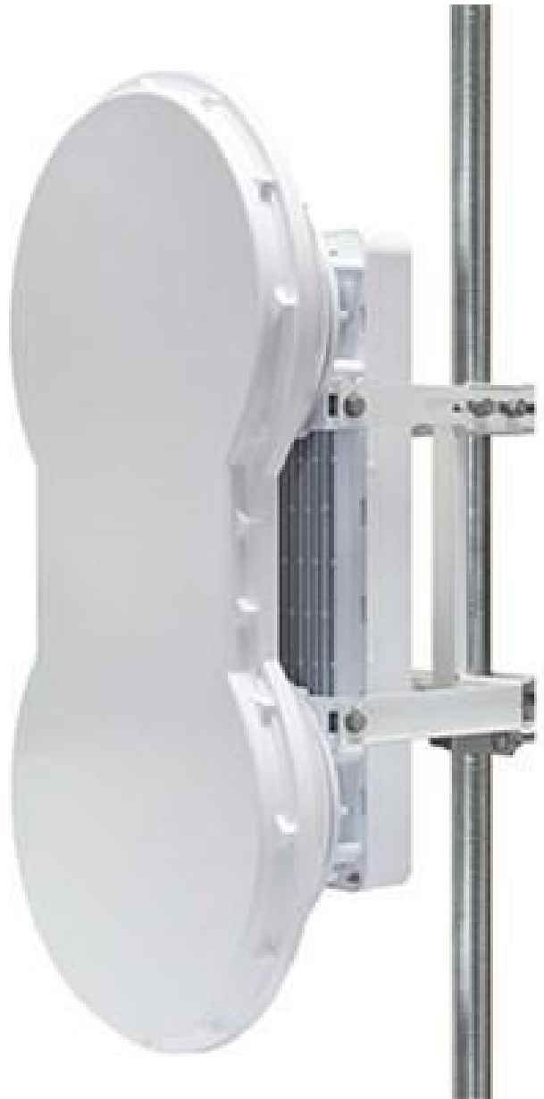
Figure 2.2. A directional wireless antenna similar to the type examined in the original point-to-point concept.
